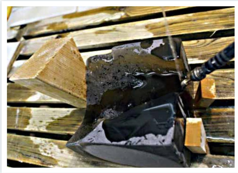
5 Wooden wedges holding the glass in place
