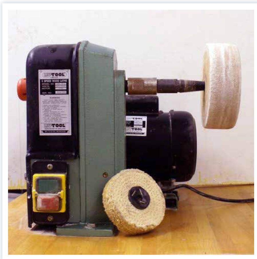
8 Wood lathe with cork and brush attachments
