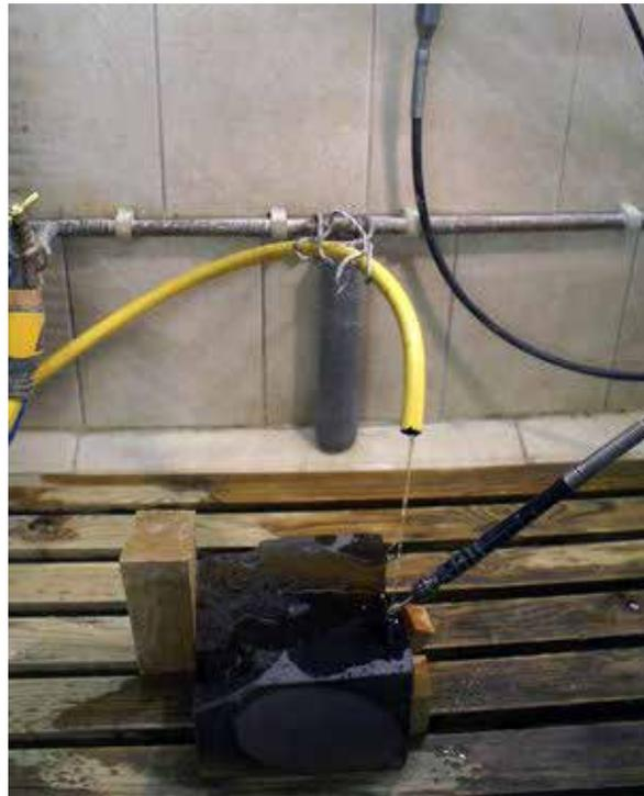
2 Slatted shelf sink with wooden wedges holding the glass, hosepipe water feed, Dremel with flexidrive and intense light source
